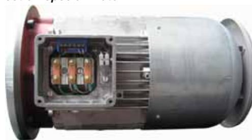
Figure G-4: Connection special motor
